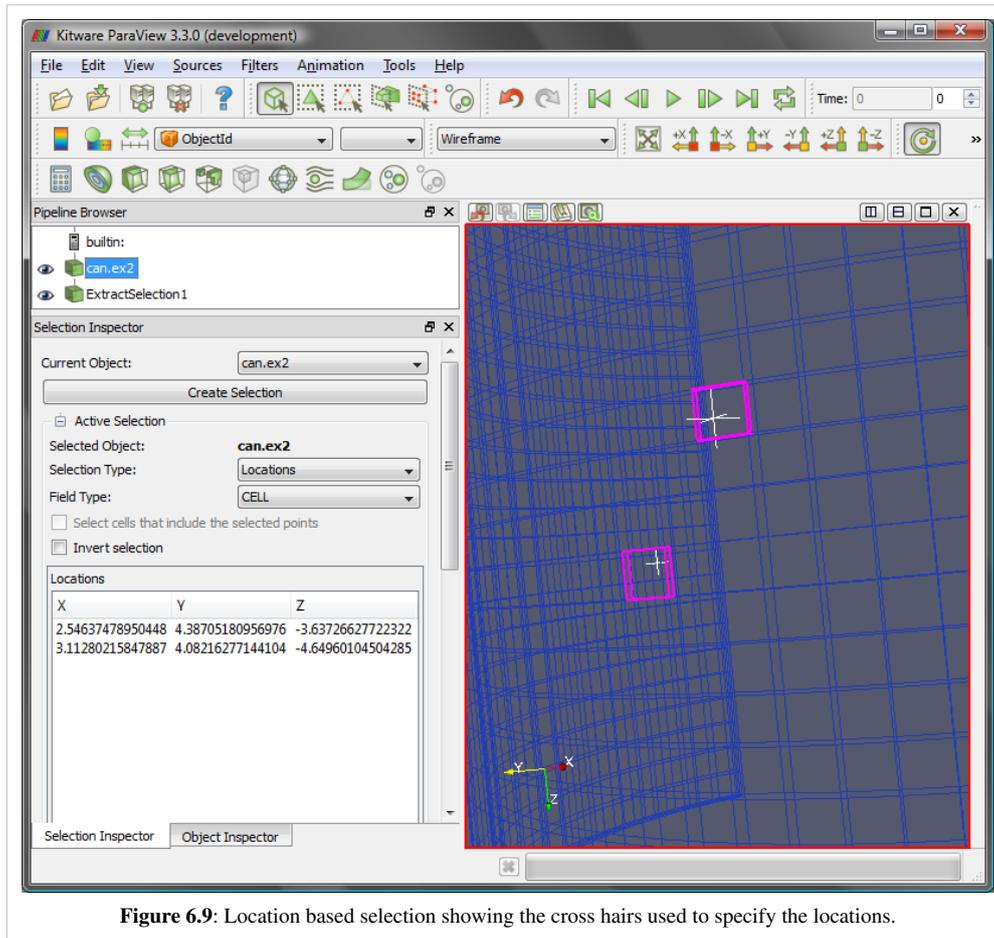
**Figure 6.9:** Location based selection showing the cross hairs used to specify the locations.
