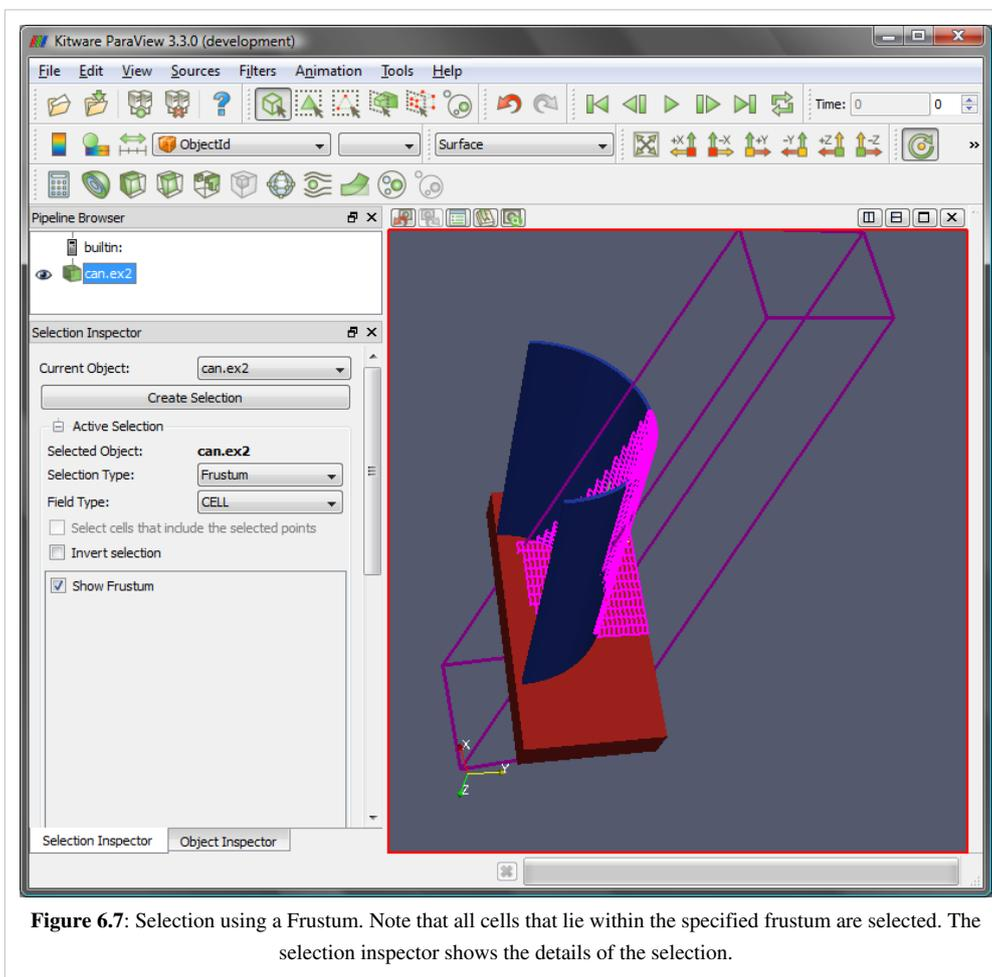
**Figure 6.7:** Selection using a Frustum. Note that all cells that lie within the specified frustum are selected. The selection inspector shows the details of the selection.
