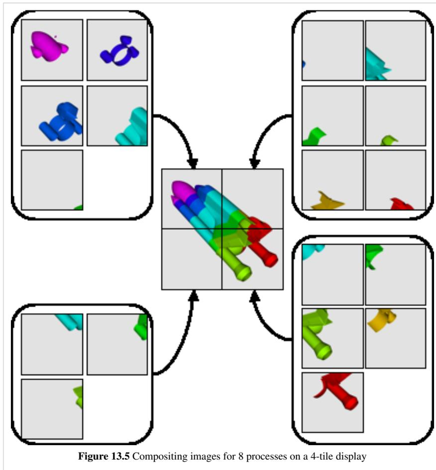
**Figure 13.5** Compositing images for 8 processes on a 4-tile display
