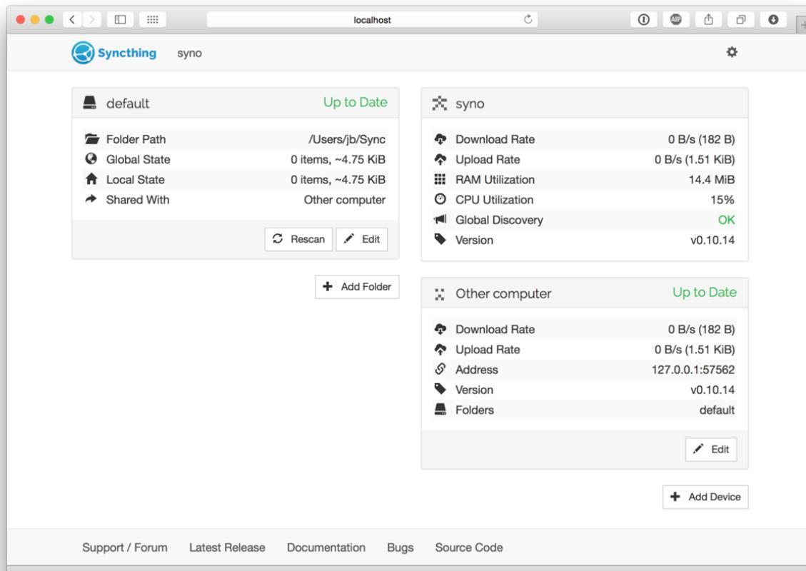
At this point the two devices share an empty directory. Adding files to the Sync directory on either device will synchronize those files to the other side. Each device scans for changes every 60 seconds, so changes can take a little over a minute to propagate to the other side. The rescan interval can be changed for each folder by clicking on a folder, clicking "Edit" and entering a new value for "Rescan Interval".
