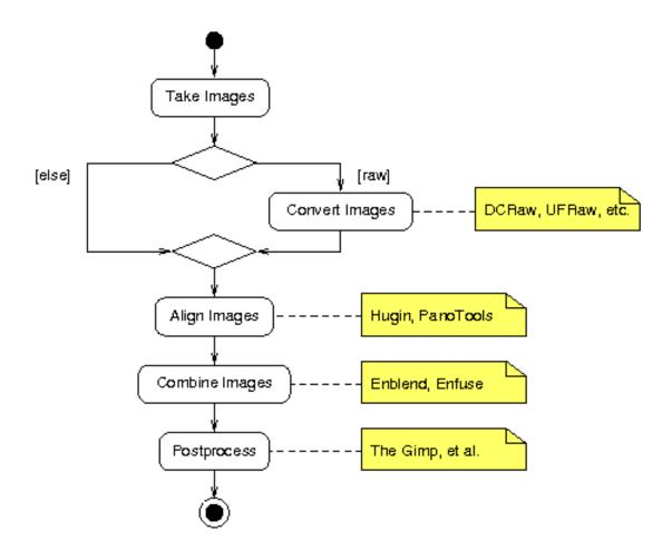
Figure 2.1: Photographic workflow with Enblend and Enfuse.
